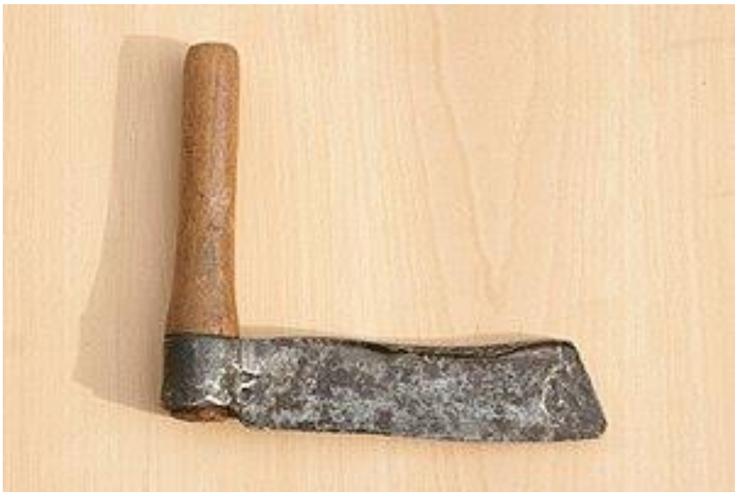
Figure 7. Archive photograph showing a complete Woodsman's Froe. Note this Froe has similar bruising on upper edge through usage.
